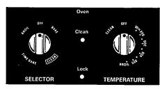
**5.** When baking is done, turn both the Temperature control and the Selector control to OFF.
