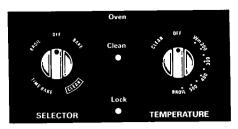
2. Turn the Selector and Temperature controls to OFF. When the Lock light goes OFF, move the Lock Lever back to the left. **DO NOT FORCE IT.** Wait until it moves easily.
