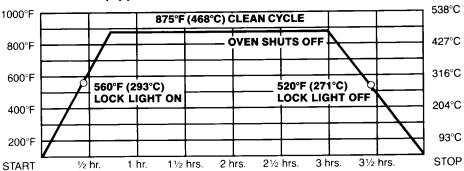
Notice that heating stops when the 3-hour setting is up, but that it takes longer for the oven to cool down enough to unlock.
