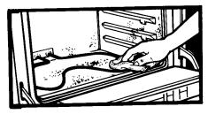
6. After the oven is cool, wipe off any residue or ash with a damp cloth. If needed, touch up spots with a soapy steel wool pad.
